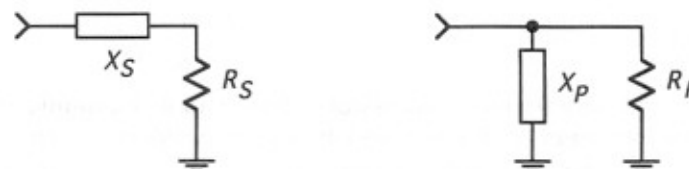
Figure 2.81 Series to parallel transformation.
