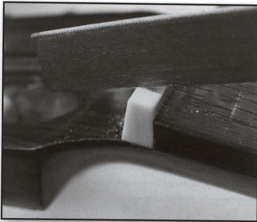
FIGURE 11.33 Shore-up the distances of the slots and cut them to the proper depth and distance. (Photo by John LeVan)
