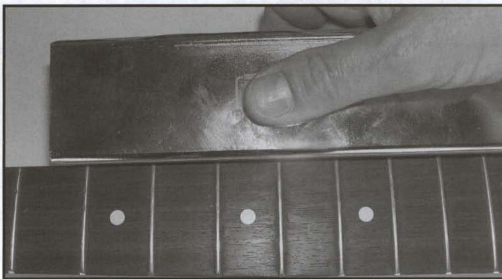
FIGURE 8.34 Avoid rolling the sandpaper over the tops of the frets; it can make them uneven. Simply skip the sandpaper along the ends of the frets. (Photo by Skip Anderson)
