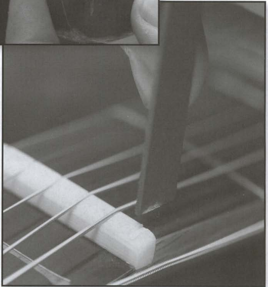
FIGURE 5.7A,B Loosely pack the slot with a like material to the nut. If the nut is bone, use bone. (Photos by Skip Anderson)
