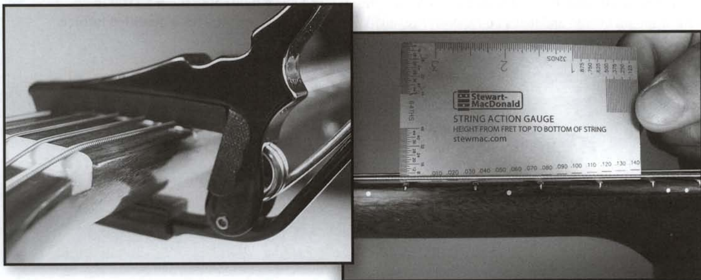
FIGURE 3.3A,B Note that the capo must be on top of the first fret, not in front of or behind it. 3.3B Hold the low E string down at the last fret and measure the greatest distance between the top of the fret to the bottom of the low E string. (Photos by John LeVan)
