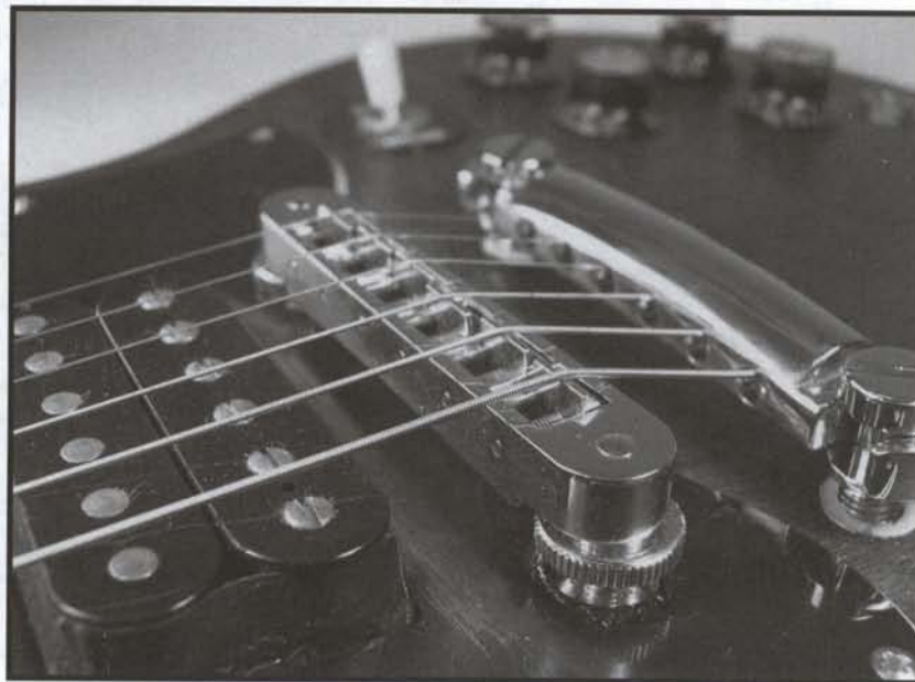
FIGURE 4.2 Tunematic® bridges are found on some electric guitars. They consist of a bridge base, bridge saddles, intonation adjustment screws, retention spring or wire, threaded inserts for the thumbwheels, and thumbwheels for height adjustment. (Photo by John LeVan)
