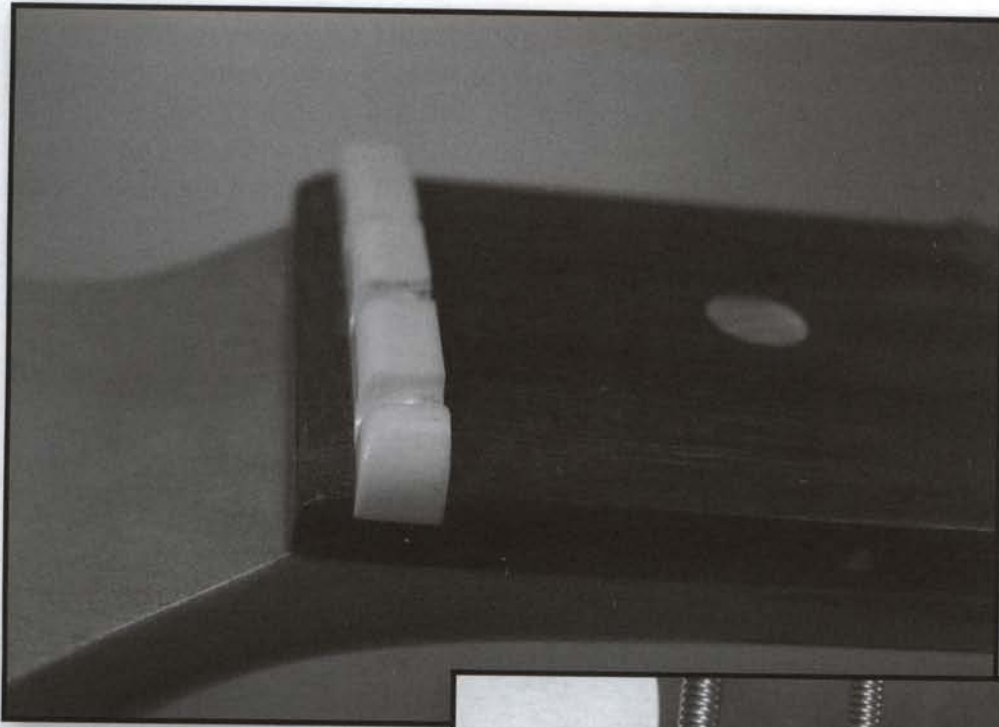
FIGURE 11.28 Carve shallow slots into the nut blank and restring. (Photo by John LeVan)
