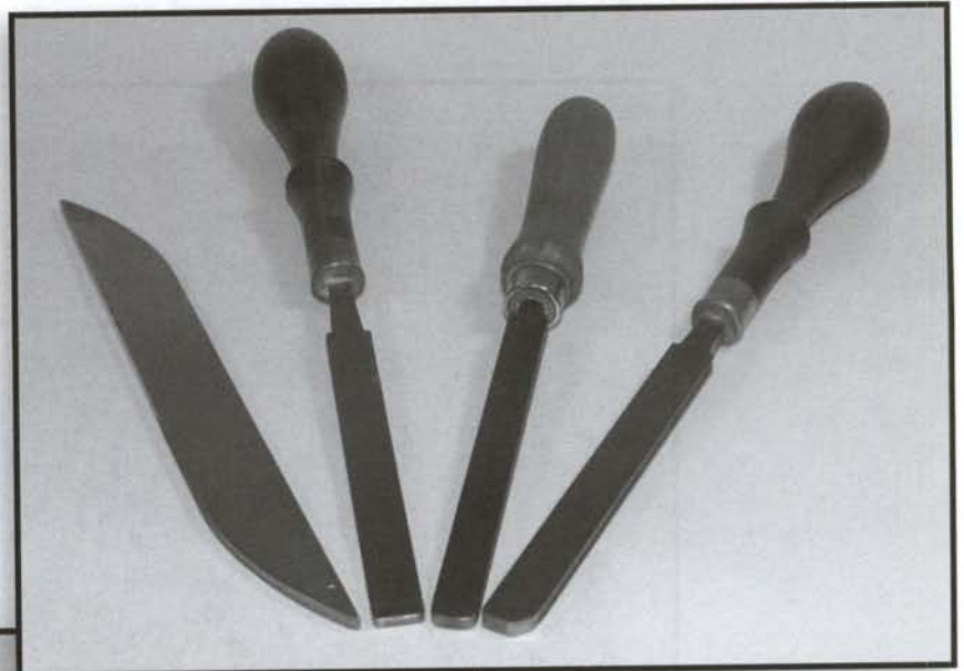
FIGURE 1.7 Fret leveling bars are made of finely milled, chrome plated bar stock and come in several sizes. The 24" and 8" leveling bars get the most use around my shop. Using self-adhesive sandpaper, the 24" is great for leveling frets, fretboards and burnishing. The 8" leveling bar is perfect for spot leveling. (Photo by Skip Anderson)
