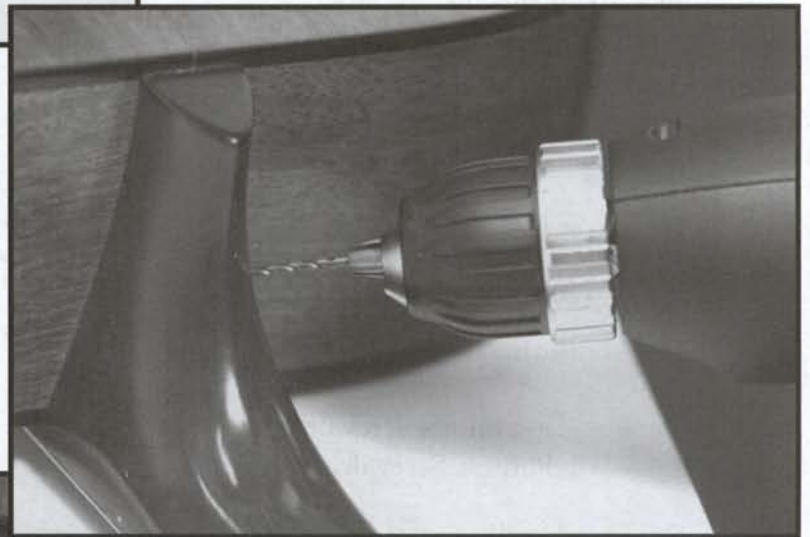
FIGURE 11.1 Location is everything. I recommend installing the button 1 1/2" below the fretboard on the treble side of the neck. If the button is installed too low on the heel, the guitar will tilt away from you when you use your guitar strap. If you place the button too high, your hand will bump it when you play on the higher frets. Once you have determined the proper location to install the strap button, gently mark it with your medium-tip Phillips screwdriver. Be careful not to slip and scratch the neck. (Photo by Skip Anderson)
