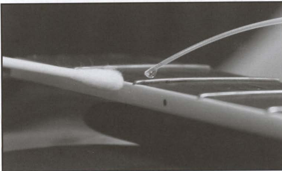
FIGURE 8.14 The ultra-thin Super Glue® will be absorbed into the wood and help hold the fret to the fretboard. This will prevent the fret from popping up again. (Photo by Skip Anderson)
