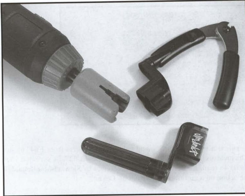
FIGURE 1.5 There are many types of string winders on the market. Varying from 99¢ to $29, this is one tool that will save you a lot of time and energy. I prefer the type that fits into a cordless drill, thus speeding up the restringing process and minimizing fatigue and the risk of developing tendonitis. (Photo by John LeVan)
