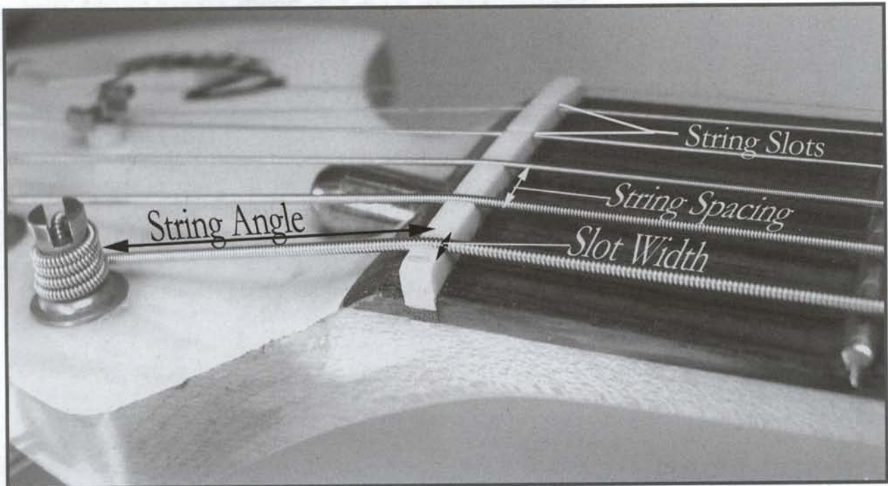
FIGURE 5.1 Here is an illustration of the string nut. (Photo by John LeVan)
