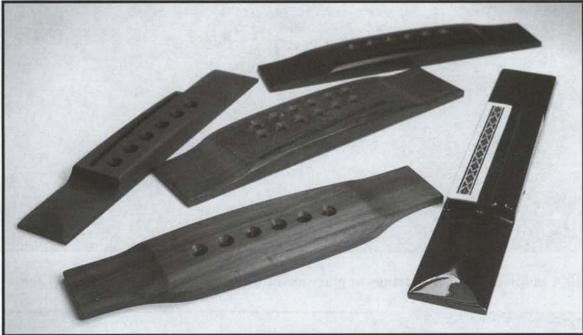
FIGURE 2.9 Acoustic guitar bridges are made from ebony, ivory, rosewood, Micarta® and even plastic. Bridge pins help to push the ball end of the strings into the bridge plate (pin plate), which is usually made from either maple or rosewood. The bridge saddle can be made from plastic, bone, ivory, graphite, brass, Micarta® or wood. Bone and ivory tend to give the most volume and dynamic range. Plastic and graphite have the least amount of volume and dynamic range. (Photo by John LeVan)
