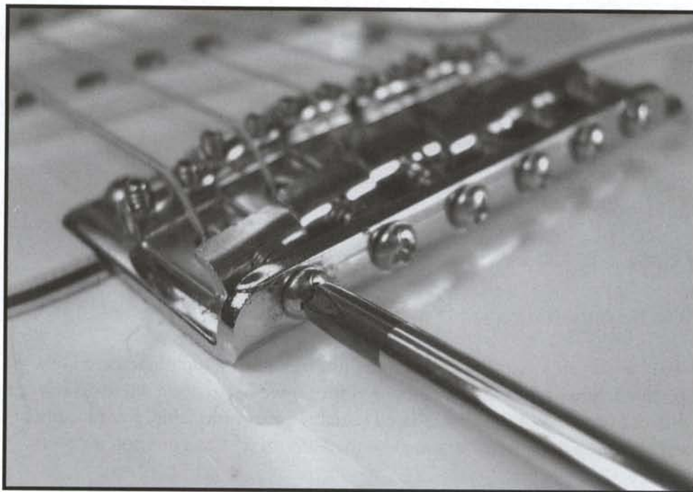
FIGURE 7.3 On an electric guitar, tighten the intonation screw if the note is sharp (#). If the note is flat (b), loosen the screw. (Photo by Skip Anderson)
