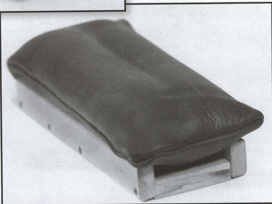
FIGURE 1.13 A bag of buckshot has several great uses other than running off an unwelcome guest. I use a 25-pound bag of no. 6 shot wrapped in leather as a neck rest when doing fretwork, setups and carving a string nut. Wrapping it in leather and then sealing it closed will help to prevent potentially harmful lead dust from escaping. (Photo by Skip Anderson)
