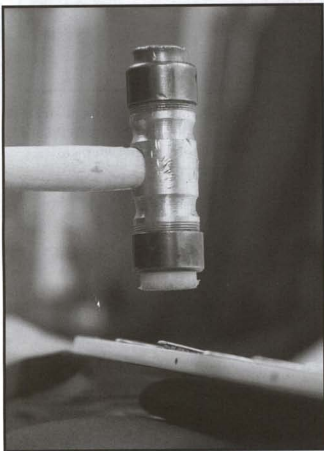
FIGURE 8.6 Fretting hammers are needed to reseat popped up fret ends and for stubborn frets that won't seat in the middle. (Photo by Skip Anderson)
