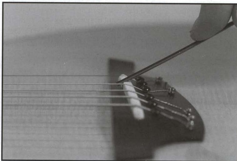
FIGURE 7.4 Use a mini flat file to carve the intonation points to the correct location on the bridge saddle. (Photo by Skip Anderson)
