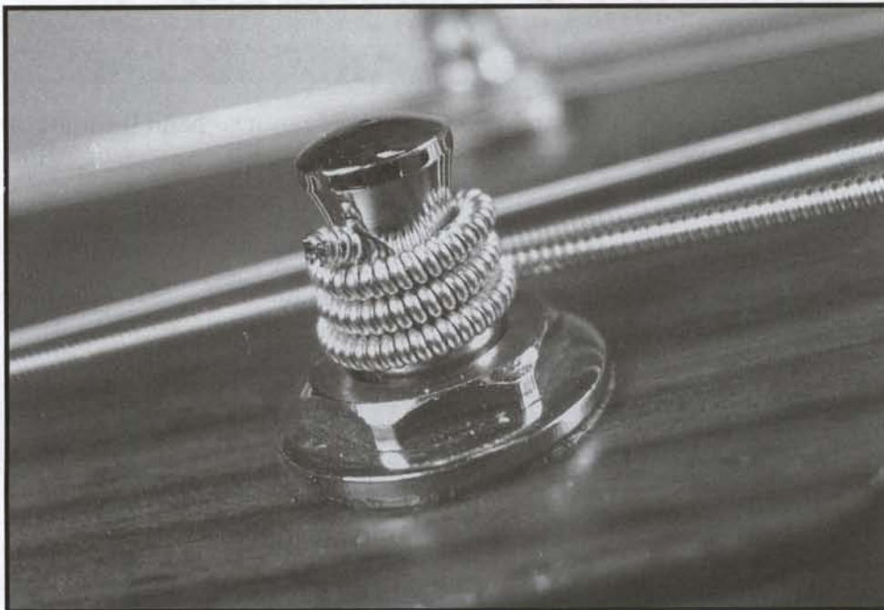
FIGURE 2.8 Wrapping the string over itself can cause string breakage and tuning problems. For the best results, wrap the string around the tuning key post in a downward direction using three or four wraps per string. (Photo by John LeVan)
