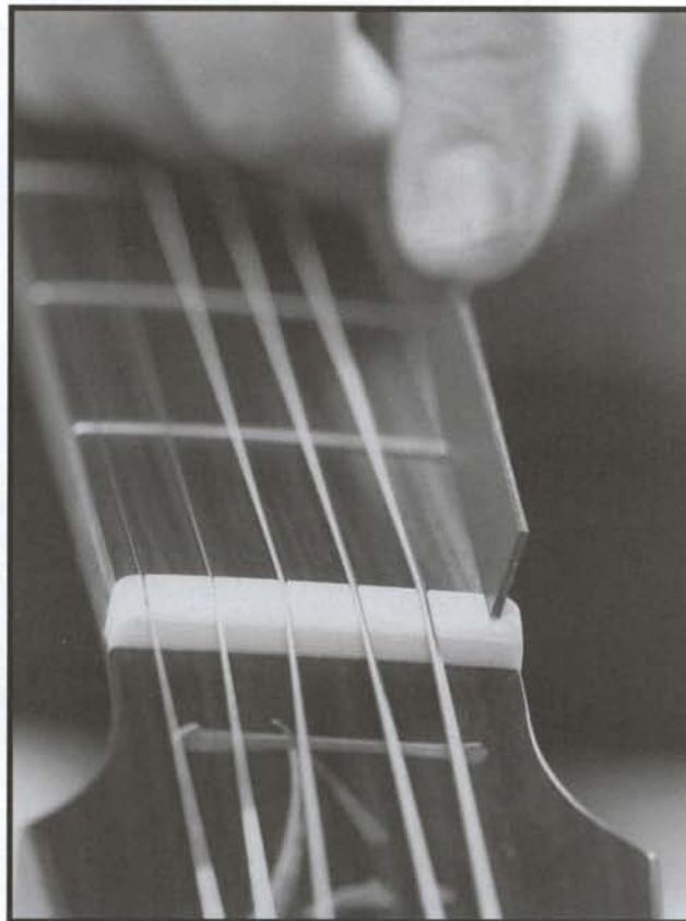
FIGURE 5.9 Re-cut the string slot to the correct width, depth and angle. (Photo by Skip Anderson)
