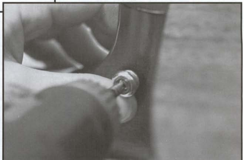
FIGURE 11.3 Using your medium-tip Phillips screwdriver, spin the handle while gently countersinking the finish around the hole. Then use a large-tip Phillips screwdriver. Don't bore into the wood too far; you only need to countersink the finish enough for the screw to clear it. This will prevent any finish from peeling up when you install the screw. (Photo by Skip Anderson)
