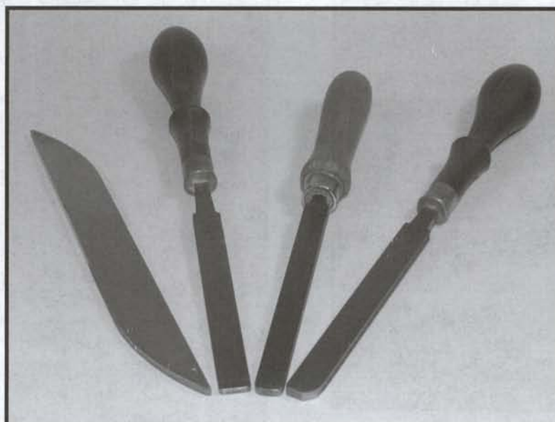
FIGURE 8.4 Recrowning files come in several sizes, shapes and cutting rasps. The half-round, dual-sized fret files work great. It is recommended to have both medium-cut and fine-cut fret files in small and medium sizes. (Photo by Skip Anderson)
