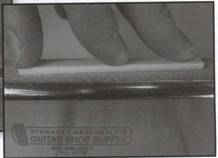
FIGURE 11.35 A,B Sand the new blank to proper size. (Photos by John LeVan)
