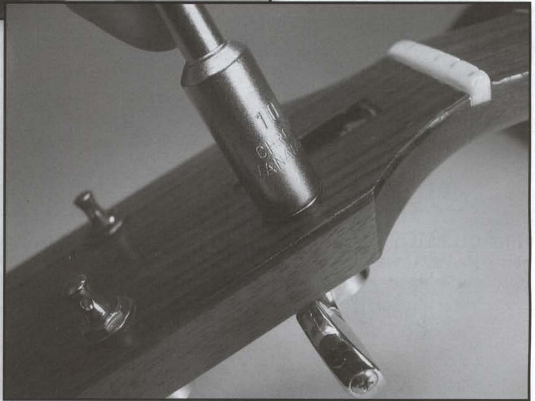
FIGURE 11.11 When installing a tuning key with a threaded collar, do not overtighten the collar. The collar can easily strip, ruining the tuning key. The collar only needs to be “finger” tight. There is no reason to torque it down with excessive pressure. (Photo by John LeVan)
