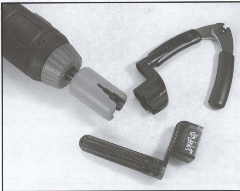
FIGURE 2.3 Electric or manual, a good string winder is essential to restringing a guitar. Likewise, a 6" pair of end cutters and an accurate guitar tuner are a must. (Photo by John LeVan)
