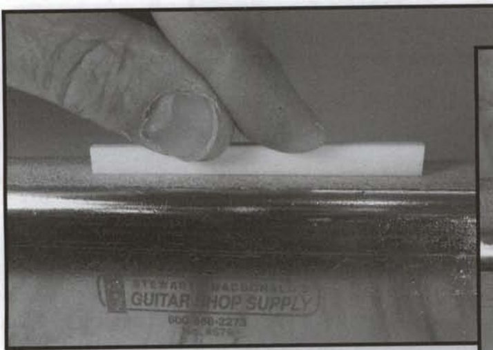
FIGURE 11.34 Use your old saddle to trace the new saddle. (Photo by John LeVan)
