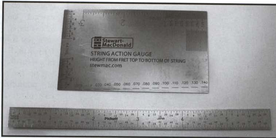
FIGURE 1.3A,B The precision scale rule is a small, six-inch, metal ruler that measures from 1/64" on up. This is important because many of the measurements in this book are in 1/64" and 1/32". Be sure that your scale has good contrast to make it easier to read. 1.3 B , An Action Gauge® (sold by Stewart-MacDonald®) is an excellent tool for measuring the action on a guitar. (Photos by John LeVan)
