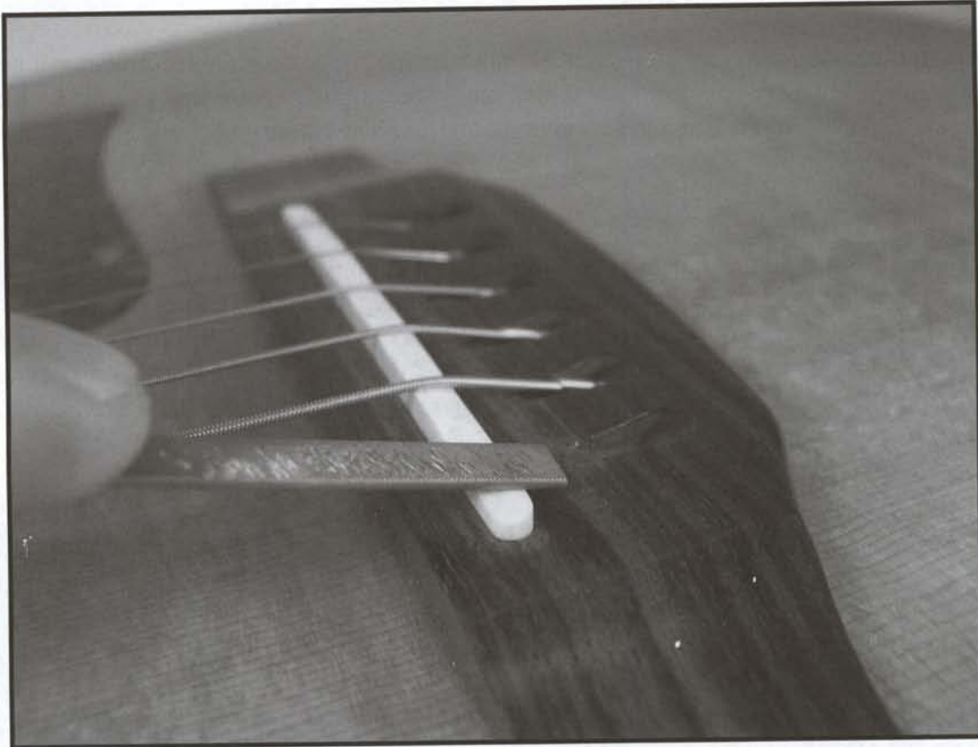
FIGURE 7.2 Be sure to carve the saddle to the correct angle with your mini flat file. Take special care not to slip and scratch the bridge or the top. A piece of cardboard or pickguard material is a wise choice to use as a shield or guard during this process. (Photo by John LeVan)
