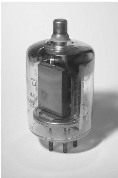
Fig. 4.35 Graphite slab anode of QV08-100 tetrode
