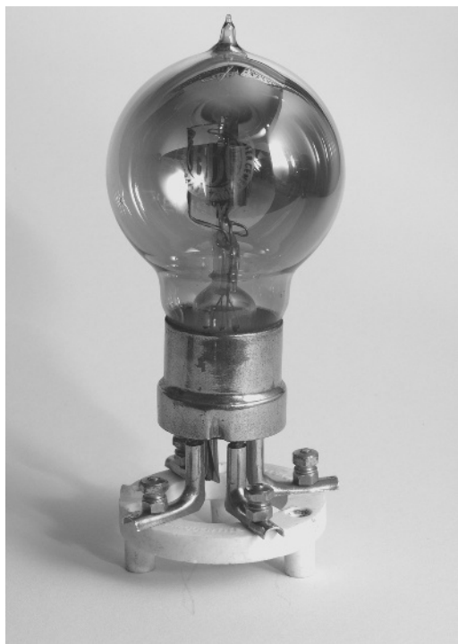
Fig. 4.24 R-type valve, note darkening of envelope. (The etched legend declares this valve to be ‘Type approved by Postmaster General BBC’)
