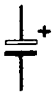
Figure E.5 Graphical symbol for an electrolytic capacitor. The positive sign is not always necessary
