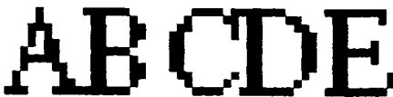
Figure A.1 Bitmapped text from a VDU display, magnified by 4, showing aliasing
