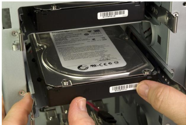
**Figure 8-14.** Slide the drive tray back into the chassis and press firmly until the spring clips snap into place
