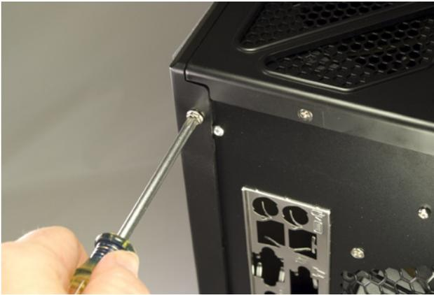
**Figure 4-4.** Remove the two screws that secure it, and then remove the left side panel
