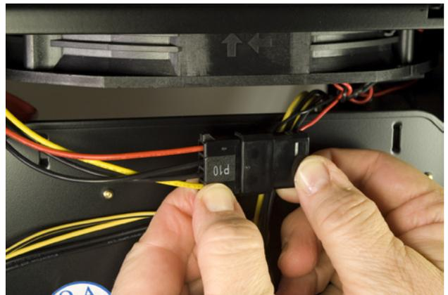
Figure 4-65. Connect power to the case fans
