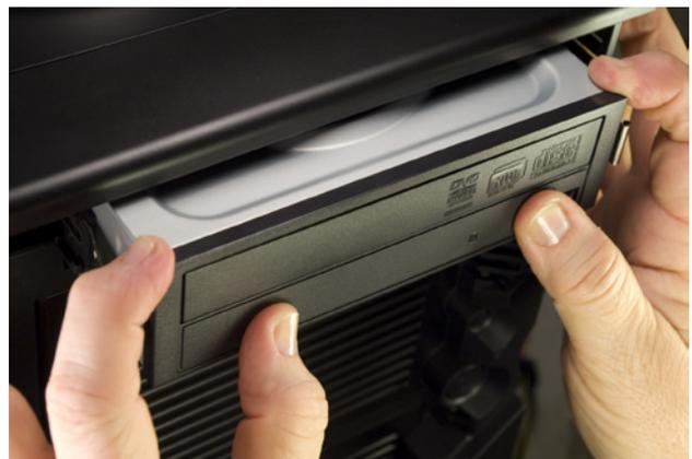
Figure 4-20. Slide the optical drive into the bay and press until both spring clips on the drive rails snap into place
