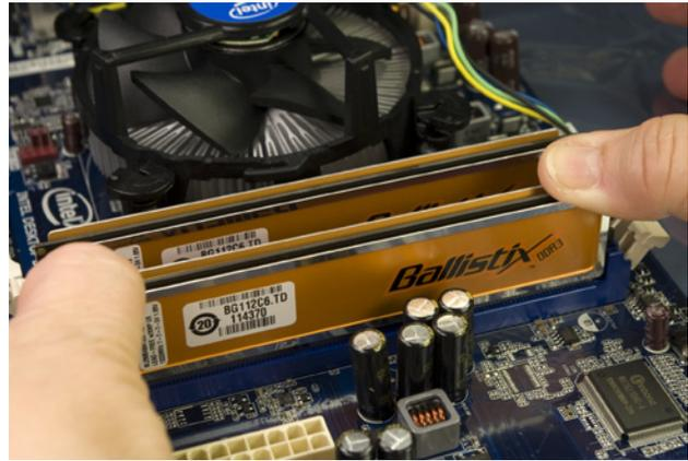
**Figure 6-19.** Press straight down with both thumbs until the module snaps into place
