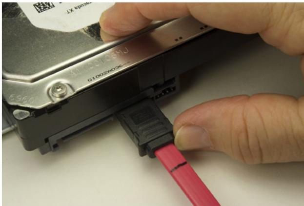
**Figure 8-13.** Connect a SATA data cable to the hard drive
