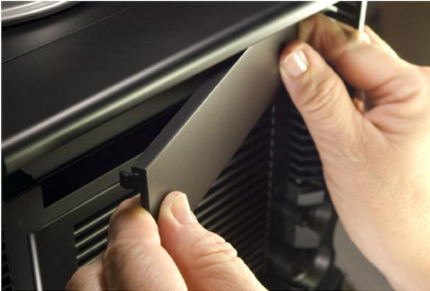
Figure 4-17. Snap out the top 5.25" drive bay bezel
