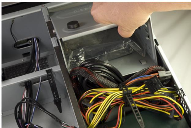
Figure 6-4. Remove the optical drive bay
