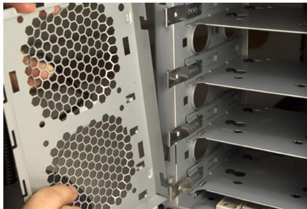
**Figure 8-8.** Lift the drive cage cover slightly to release it, and set it aside
