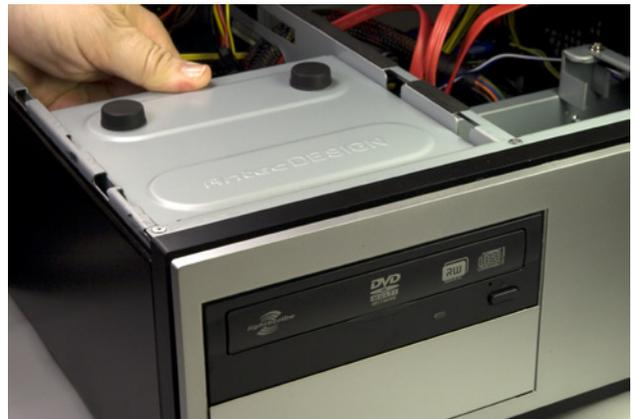
**Figure 6-36.** Slide the optical drive cage into the chassis
