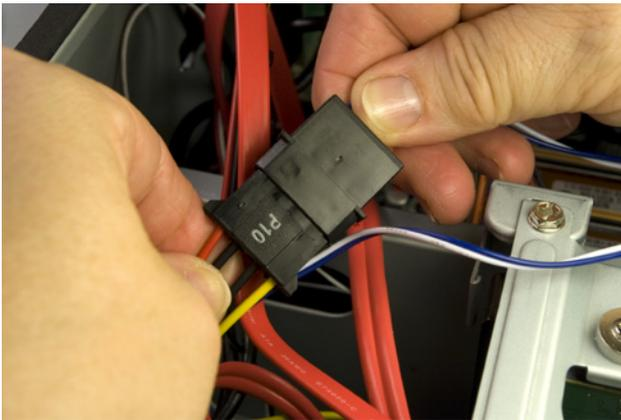
Figure 6-58. Connect power to the power LED
