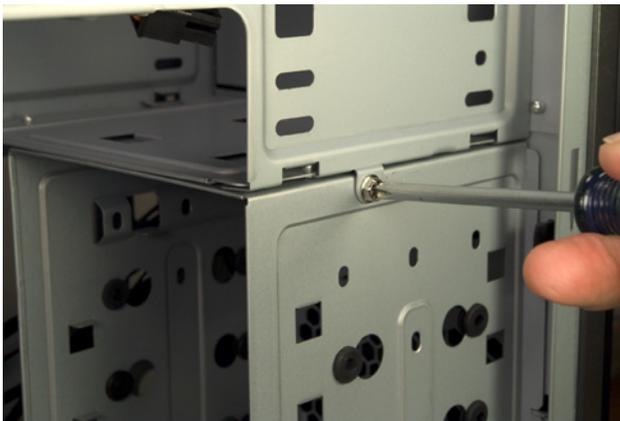
**Figure 3-5.** Remove the screw that secures the side of the 3.5" internal drive bay to the 5.25" drive bay above it
