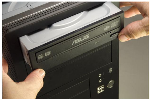
**Figure 3-11.** Slide the optical drive into the drive bay until its bezel is flush with the case bezel
