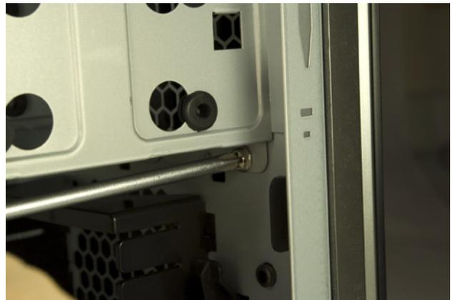
**Figure 3-6.** Remove the two screws that secure the bottom of the 3.5" internal drive bay to the front of the chassis
