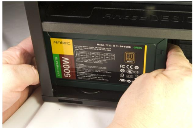
**Figure 4-7.** Slide the power supply into position
