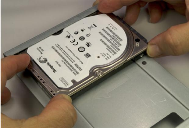
Figure 7-25. Orient the hard drive correctly, and slide it into the HDD tray
