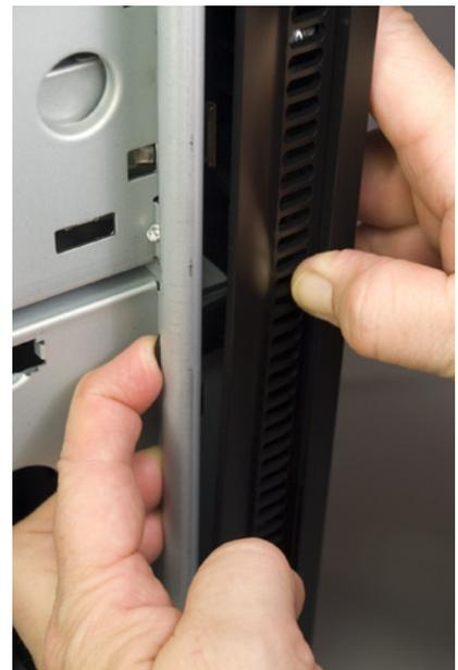
**Figure 8-4.** Release the three latching tabs that secure the front bezel to the chassis frame
