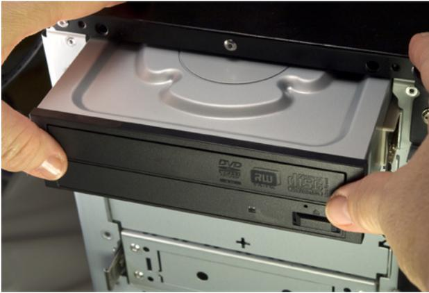
**Figure 8-45.** Slide the drive into the chassis and press until it latches
