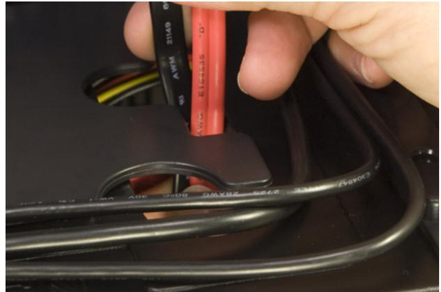
**Figure 4-53.** Route the two SATA data cables from the Easy SATA through the bulkhead and into the upper chamber
