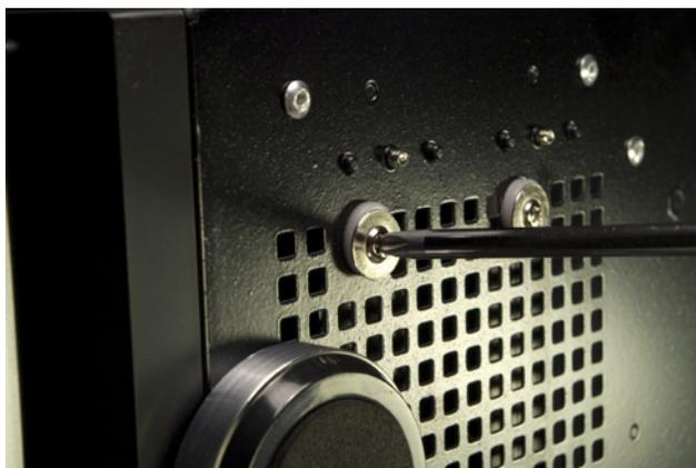
**Figure 6-50.** Secure the second hard drive to the chassis by driving two hard drive mounting screws through the bottom of the case and into the drive
