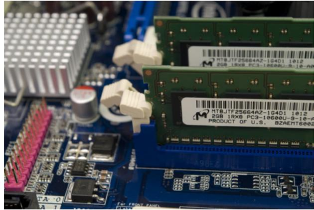
Figure 4-35. Verify that the DIMMs are fully seated and the latching posts are in the latched position
