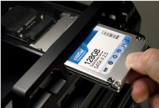
**Figure 5-66.** Slide the SSD boot drive into the top 2.5" drive bay (but not this way)
