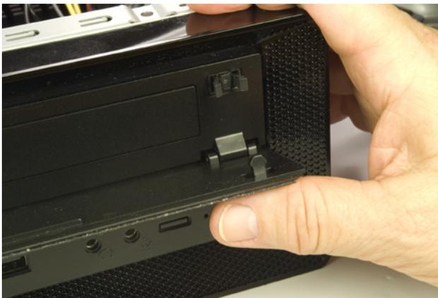
Figure 7-29. Release the optical drive bezel and allow it to pivot down
