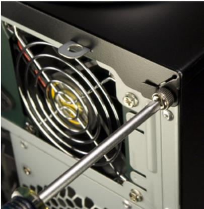
Figure 3-2. Remove the two thumbscrews that secure the top panel
