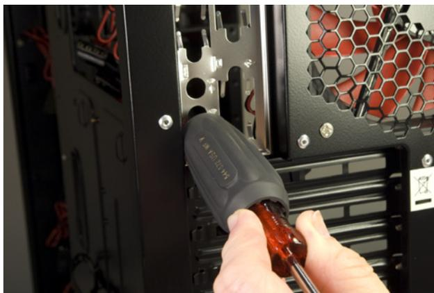
Figure 5-10. Use a tool handle to snap out the stock I/O shield
