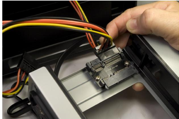
**Figure 4-49.** Connect power to the Easy SATA unit
