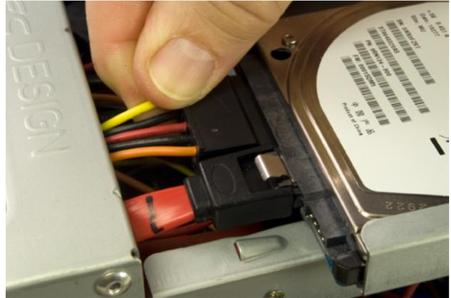
**Figure 7-36.** Connect the SATA data and power cables to the hard drive
