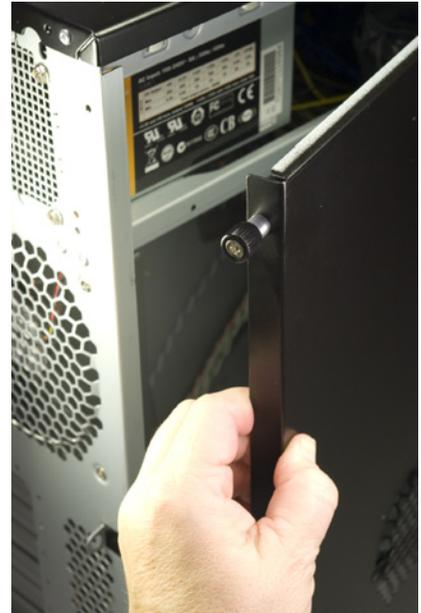
**Figure 8-3.** Swing the side panel out and remove it from the case
