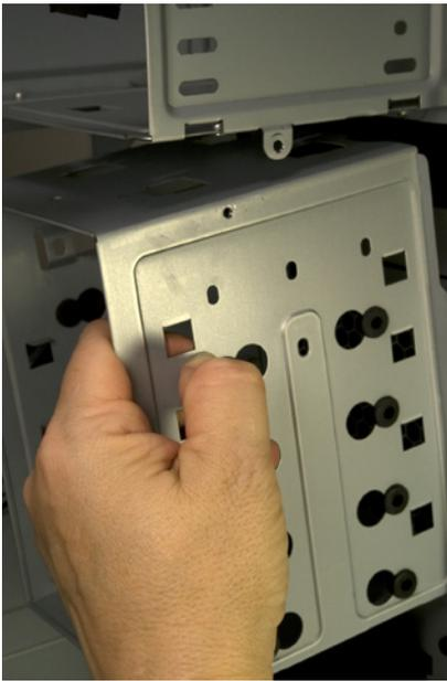
**Figure 3-7.** Slide the 3.5" internal drive bay slightly toward the rear of the case and lift it out
