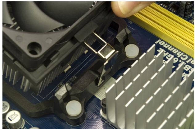
**Figure 3-20.** Hook the free-floating metal bracket over the black plastic tab on the processor socket
