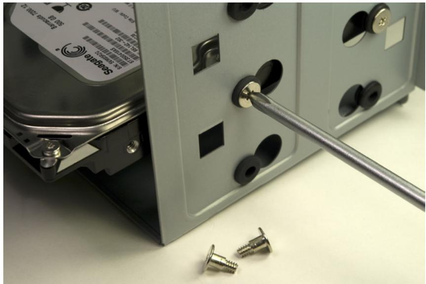
**Figure 3-8.** Slide the hard drive into the internal drive bay and secure it with four hard drive mounting screws
