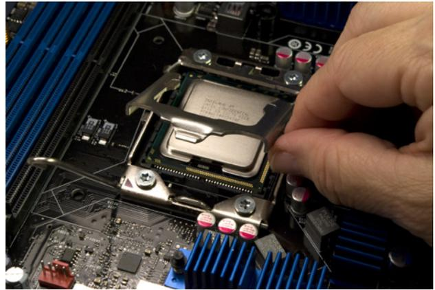
**Figure 5-26.** Lower the load plate into closed position
