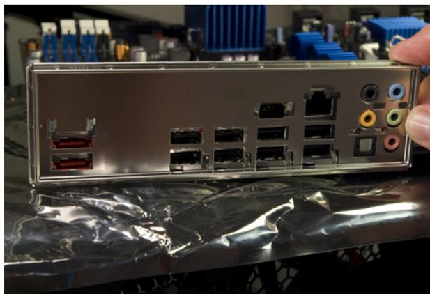
Figure 5-11. Compare the custom I/O shield with the motherboard back-panel connectors
