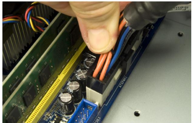
**Figure 8-36.** Connect the 24-pin main ATX power cable from the power supply to the motherboard
