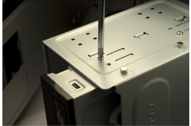
**Figure 6-34.** Secure the optical drive to the bay with four screws
