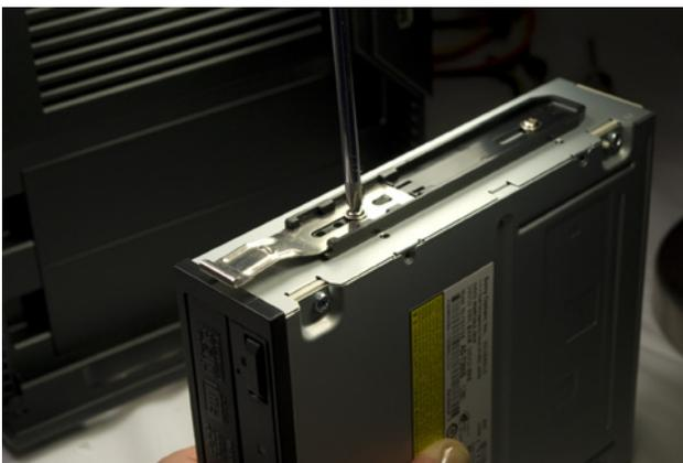
Figure 4-19. Use two screws to secure the drive rail to the optical drive
