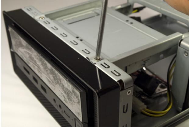
**Figure 7-4.** Remove the three Phillips screws that secure the drive tray to the frame
