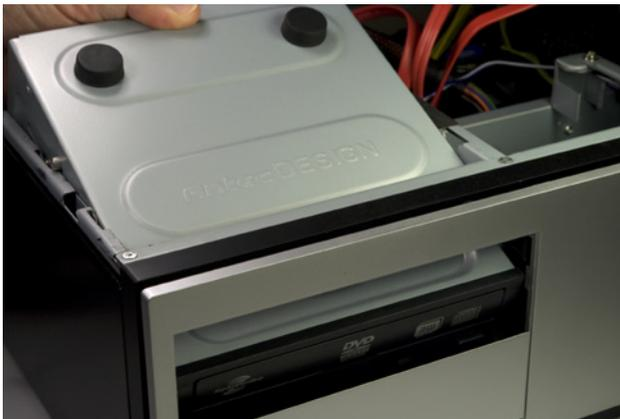
**Figure 6-35.** Slide the optical drive cage into the case
