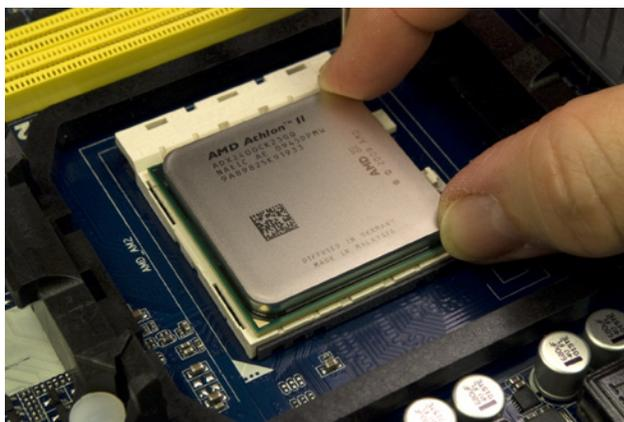
Figure 8-18. Orient and align the processor properly with the socket and then drop it into place
