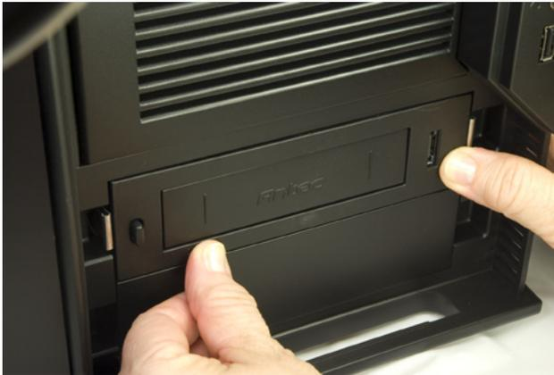
**Figure 4-52.** Press the Easy SATA frame into the drive bay until the spring clips snap into place
