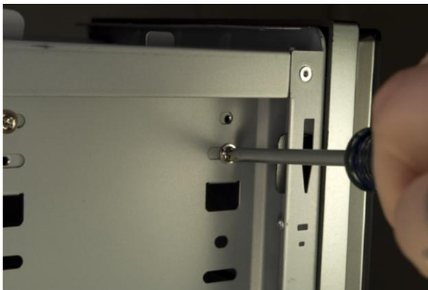
**Figure 3-12.** Use at least four screws (two per side) to secure the optical drive to the chassis
