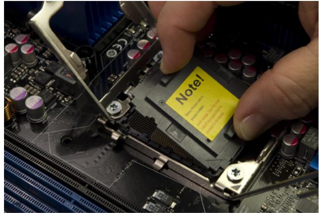
Figure 5-24. Remove the socket cover
