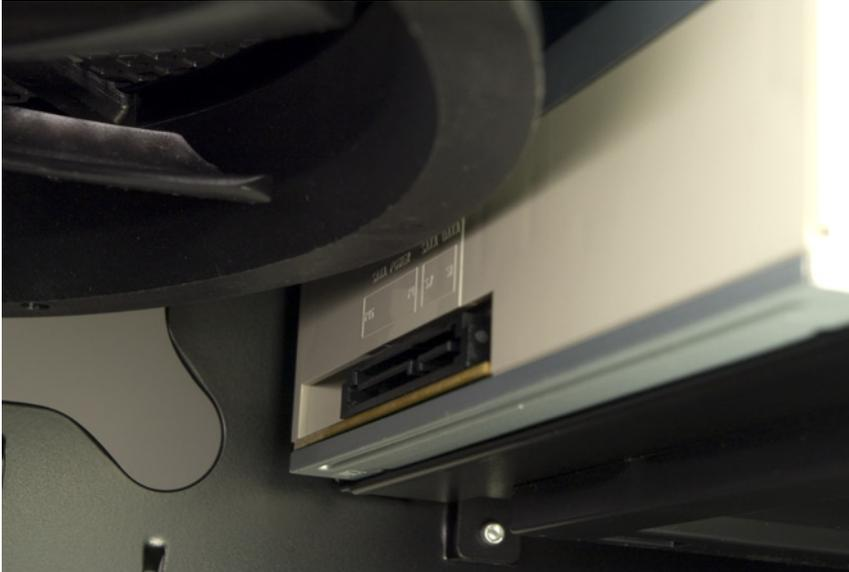
**Figure 4-21.** Verify that the top fan assembly doesn't interfere with the optical drive
