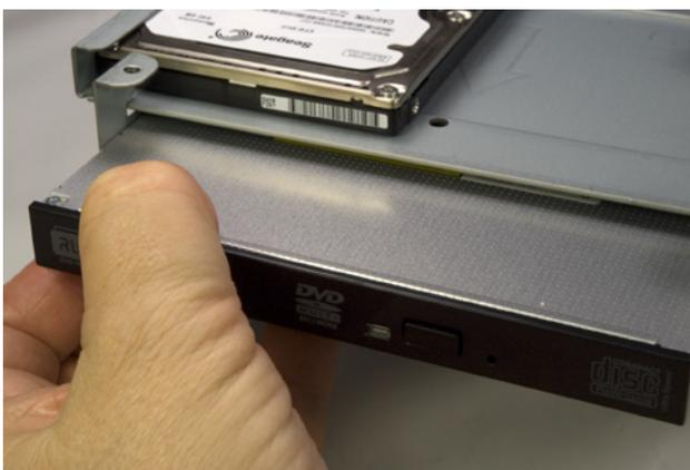
Figure 7-31. Slide the optical drive into the bay
