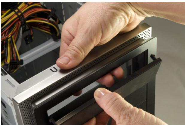
**Figure 3-10.** Working from inside the case, press the top plastic drive bay bezel until it snaps out
