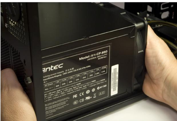
**Figure 5-19.** Slide the power supply into position
