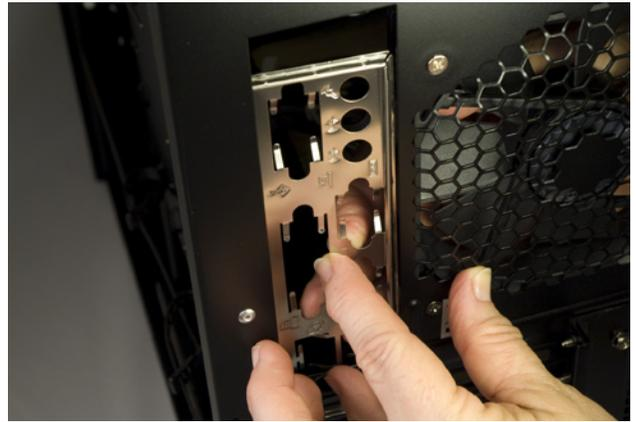
**Figure 4-5.** Remove and discard the I/O shield supplied with the case
