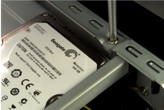
**Figure 7-35.** Reinstall the drive tray assembly and secure it with three screws
