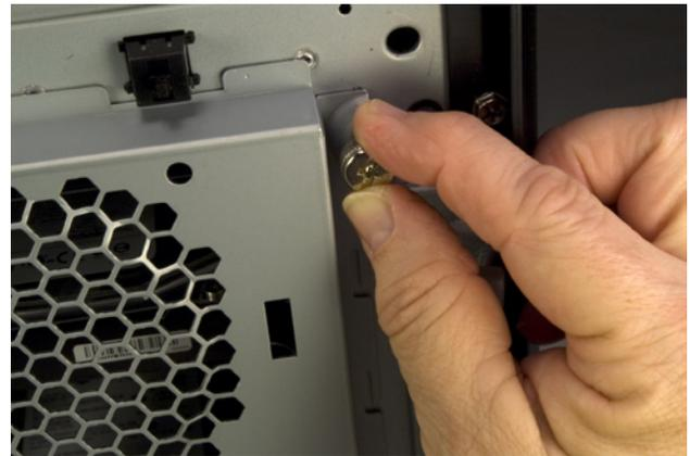
Figure 8-16. Reinsert the thumbscrews to secure the drive bay cover
