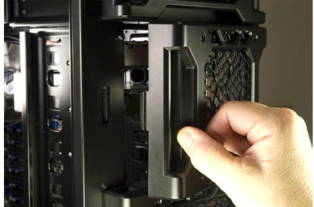
Figure 5-56. Close and latch the drive bay door
