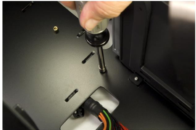
**Figure 4-38.** Install any missing standoffs needed to support the motherboard
