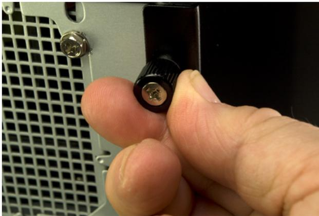
**Figure 8-2.** Loosen both captive thumbscrews on the rear of the left side panel
