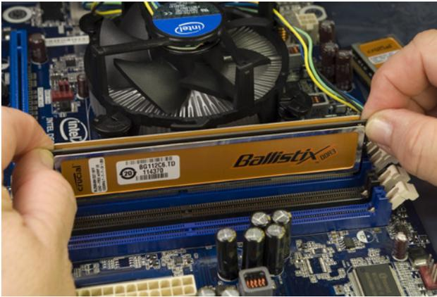
**Figure 6-18.** Position the memory module with the notch aligned with the socket tab
