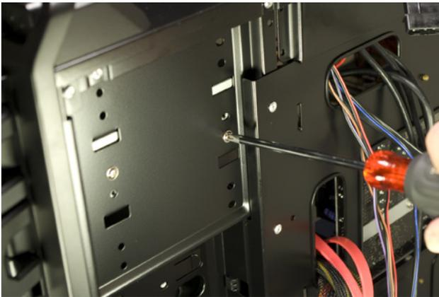
**Figure 5-63.** Secure the optical drive with at least two screws per side
