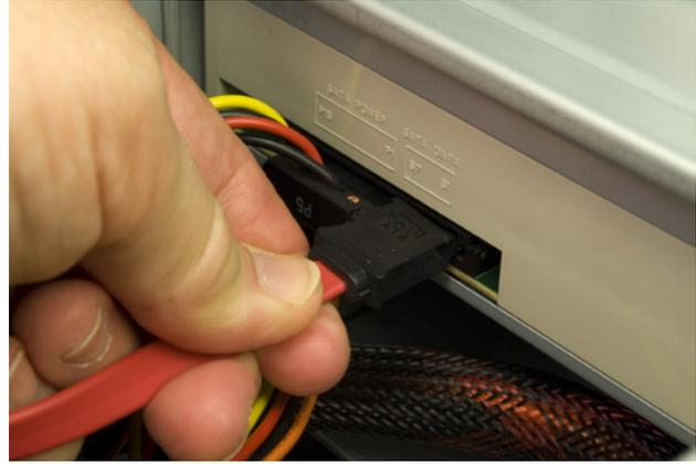
Figure 6-38. Connect the SATA data cable to the optical drive
