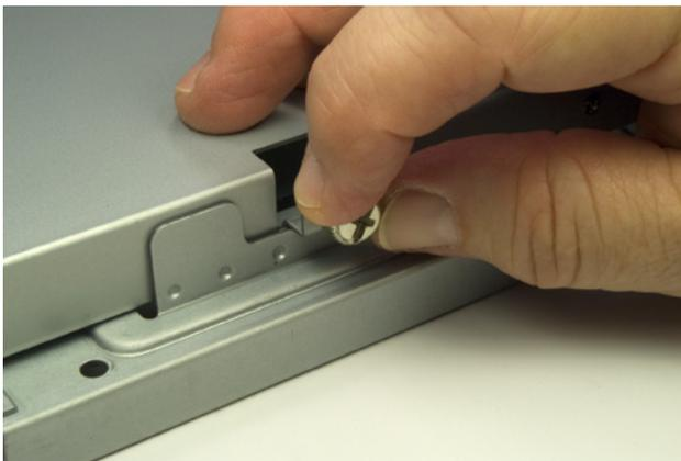
**Figure 7-23.** Remove the thumbscrew that secures the HDD tray to the drive tray assembly
