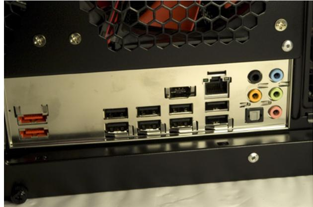
**Figure 5-43.** Verify that none of the back-panel I/O ports are fouled by the grounding tabs on the I/O shield
