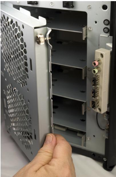
**Figure 8-7.** Swing the drive cage cover open
