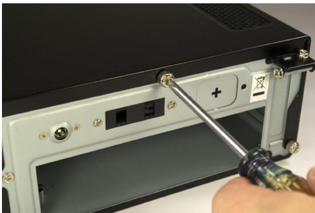
Figure 7-2. Remove the three thumbscrews that secure the cover
