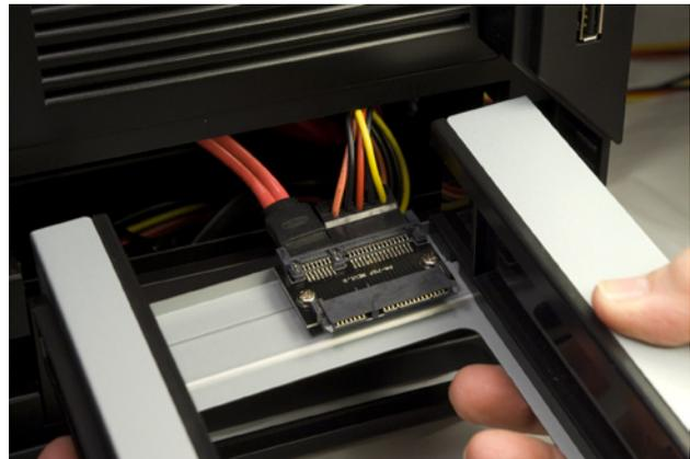
**Figure 4-51.** Slide the Easy SATA unit into the drive bay
