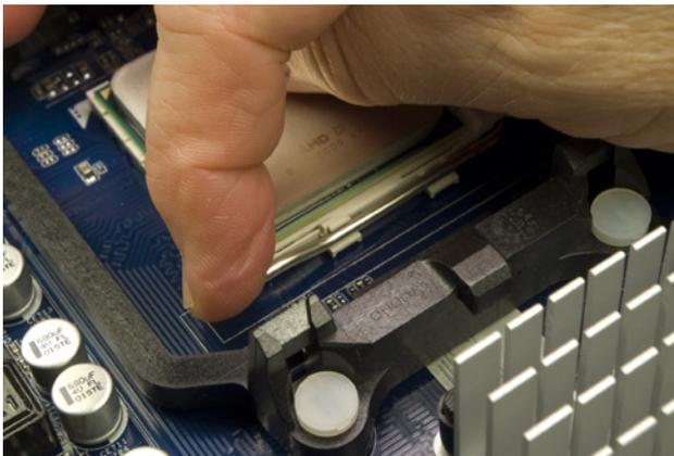
**Figure 3-19.** Press the cam lever down and snap it into place under the plastic locking tab on the processor socket
