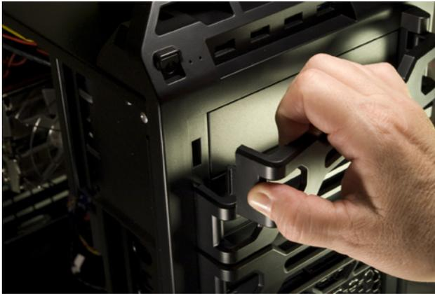
**Figure 5-59.** Press in on the left side to release the catch, and then swing open the door covering the top 5.25" drive bay
