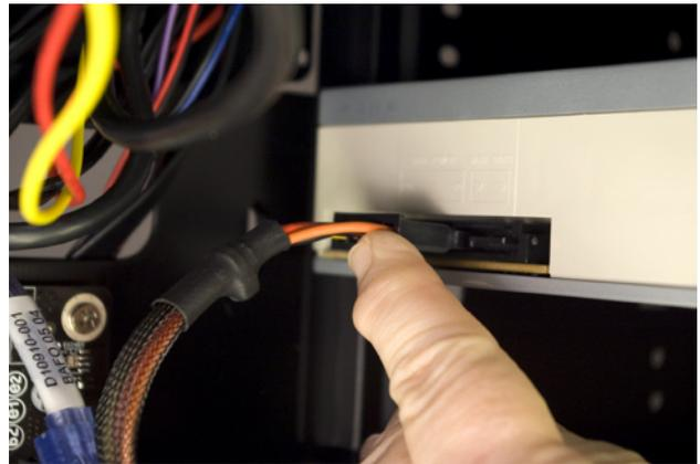
**Figure 5-64.** Connect power to the optical drive
