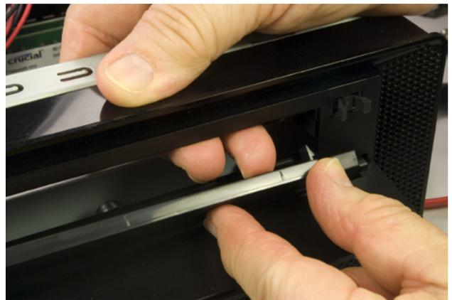
Figure 7-30. Press gently from inside the case to pop out the drive bay face plate
