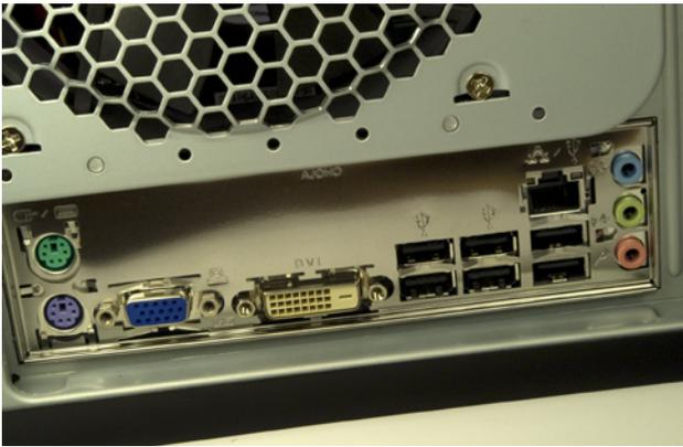
**Figure 8-33.** Verify that none of the grounding tabs on the I/O shield have fouled motherboard I/O port connectors
