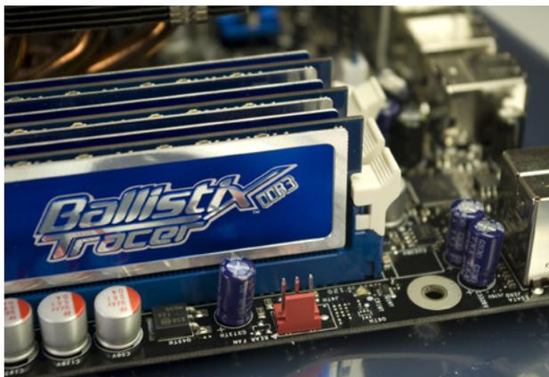
Figure 5-37. Verify that the pivoting latches have locked each memory module into place
