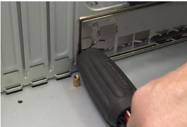
**Figure 8-30.** Position the I/O shield and press gently until it snaps into position
