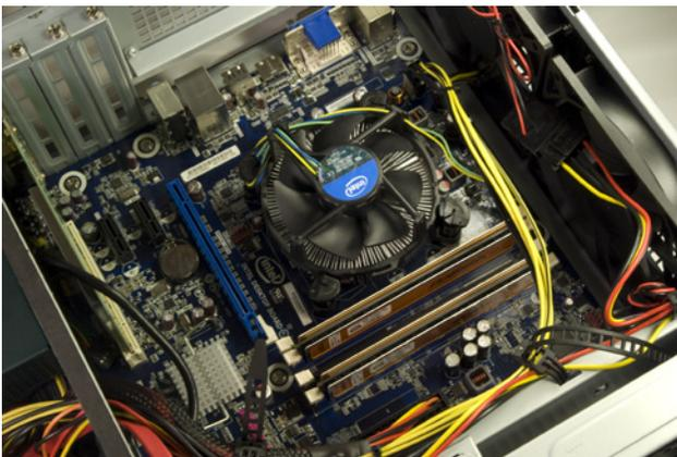
Figure 6-62. The final system, with cables dressed
