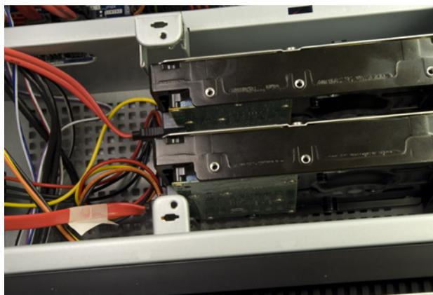
**Figure 6-51.** Both hard drives properly mounted
