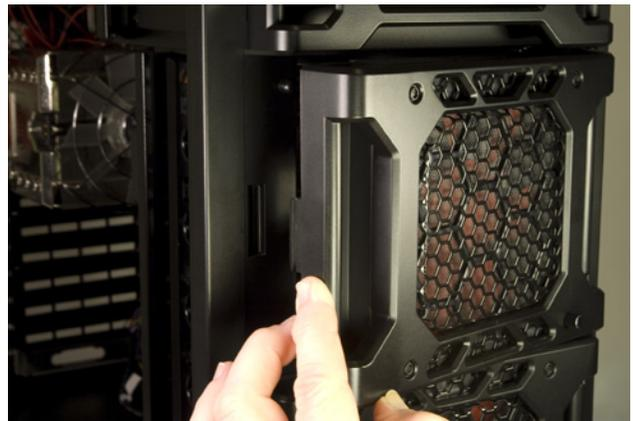
**Figure 5-54.** Unlatch the drive bay door by pressing in on the left side, and then swing the door open
