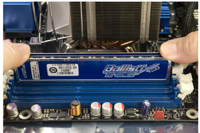
Figure 5-36. Press down firmly to seat the memory module in the socket
