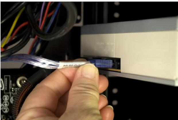
**Figure 5-65.** Connect the SATA data cable to the optical drive
