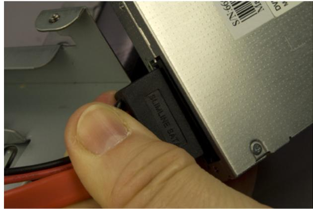
Figure 7-34. Connect the Slimline SATA adapter to the optical drive
