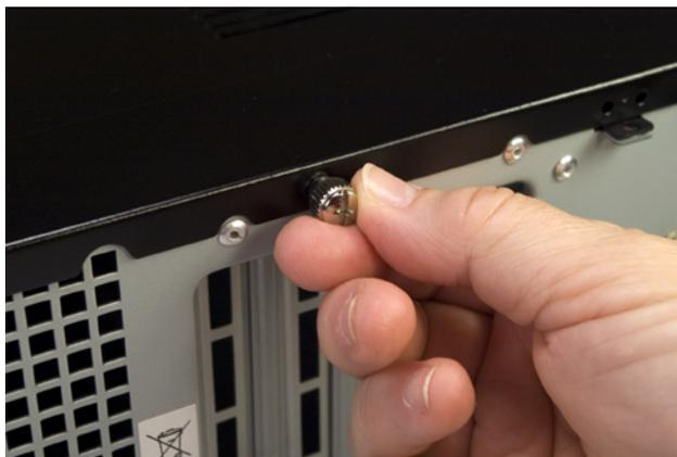
Figure 6-2. Remove the thumbscrew that secures the top panel
