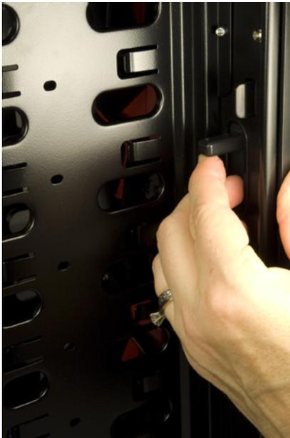
**Figure 5-53.** Slide the drive bay door locking lever up to the unlocked position
