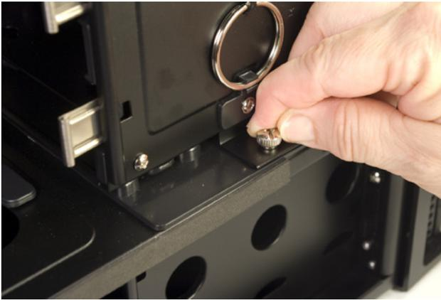
Figure 4-10. Remove the thumbscrews that secure the drive cages
