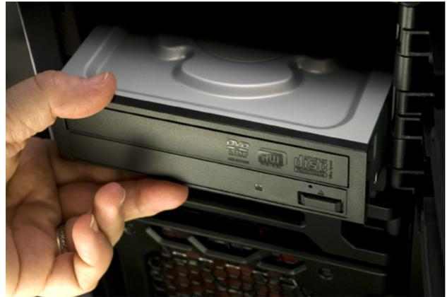
**Figure 5-62.** Slide the optical drive into the bay
