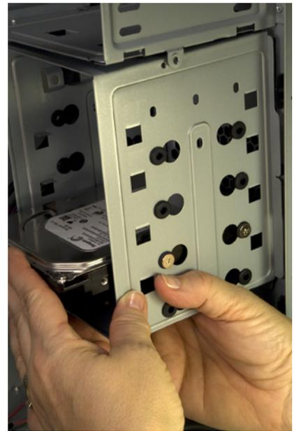
**Figure 3-9.** Slide the internal drive bay back into place and secure it with the three screws you removed earlier
