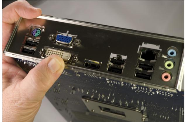
Figure 6-7. Compare the custom I/O shield with the I/O panel of the motherboard
