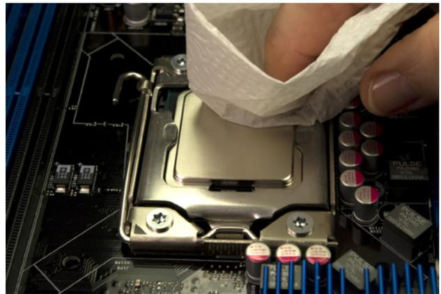
**Figure 5-28.** If necessary, use a clean paper towel to polish the processor surface and remove contaminants
