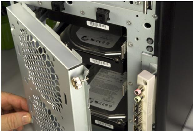
Figure 8-15. Align the pins on the drive bay cover with the sockets in the chassis and lower the drive bay cover back into place
