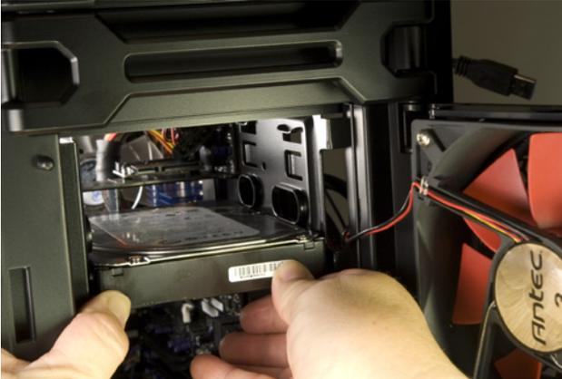
Figure 5-55. Slide the hard drive into the drive bay
