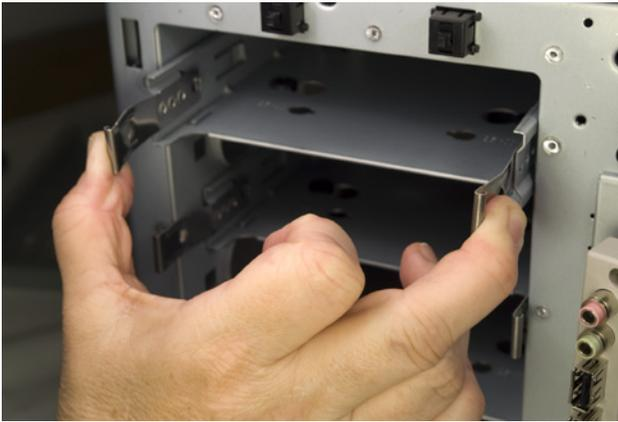
**Figure 8-9.** Remove drive trays by squeezing both metal clips and pulling the drive tray straight out of the chassis
