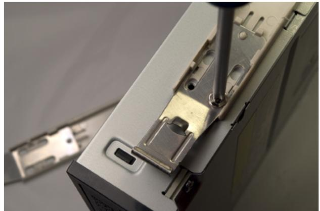
Figure 8-44. Install drive rails on both sides of the optical drive
