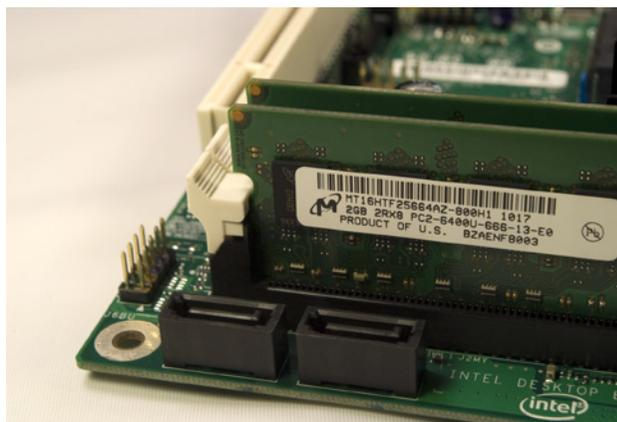
Figure 7-11. Make sure the latches engage the notches on the DIMM to lock the DIMM into place
