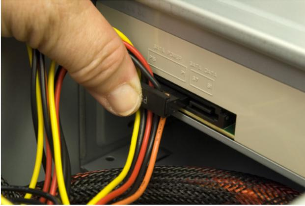
Figure 6-37. Connect a SATA power cable to the optical drive
