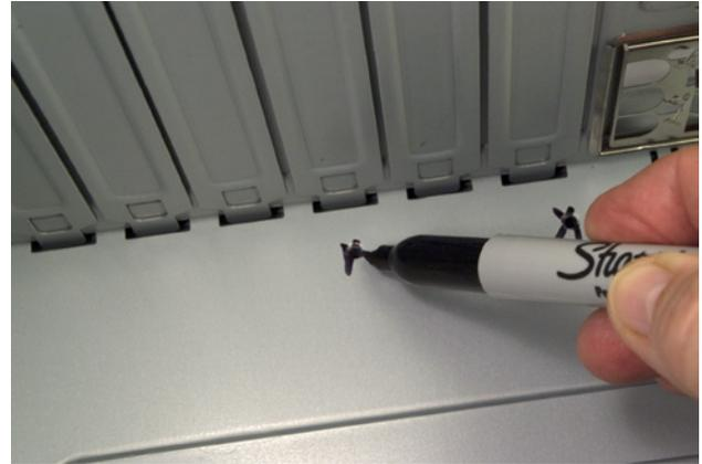
Figure 3-15. Locate and mark the proper positions for standoffs to be installed
