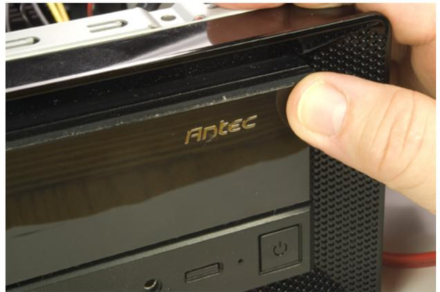
Figure 7-28. Press gently on the optical drive bezel to unlatch it
