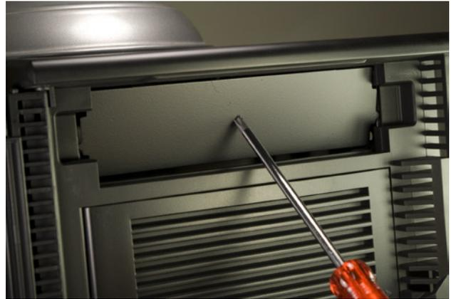
Figure 4-18. Twist the metal RF shielding plate until it snaps free
