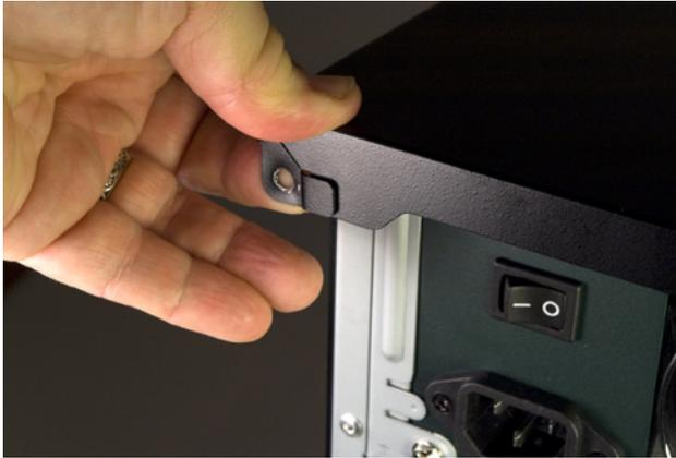
**Figure 3-3.** Slide the top panel to the rear to release it
