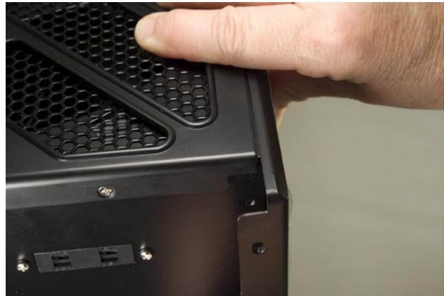
**Figure 4-3.** Slide the right side panel back an inch or so and remove it
