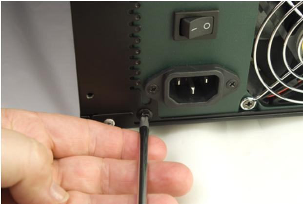
Figure 4-8. Secure the power supply to the case with four screws
