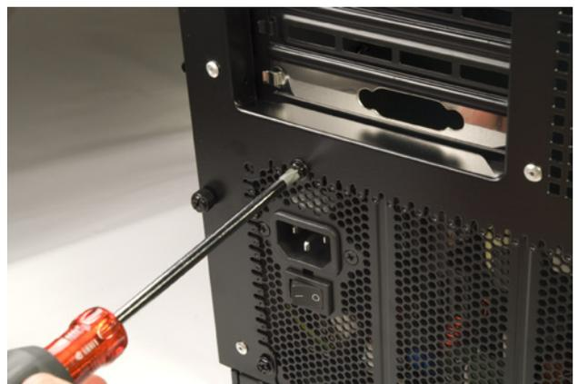
**Figure 5-20.** Secure the power supply to the chassis with the four provided screws
