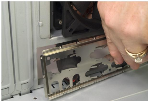
**Figure 3-13.** Remove the I/O shield supplied with the case
