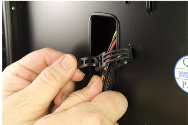
Figure 4-9. Route cables along the outer right side of the chassis and through the cutouts
