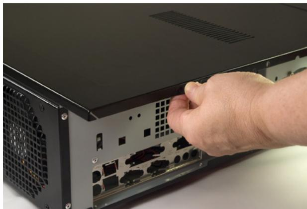
Figure 6-3. Slide the top panel to the rear and lift it off
