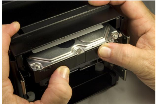
**Figure 4-15.** Slide the drive tray into the drive cage until the spring clips snap into place
