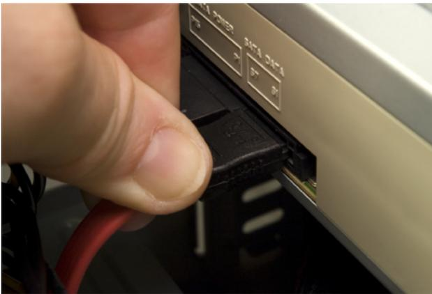
Figure 3-38. Connect SATA data cable 1 to the optical drive
