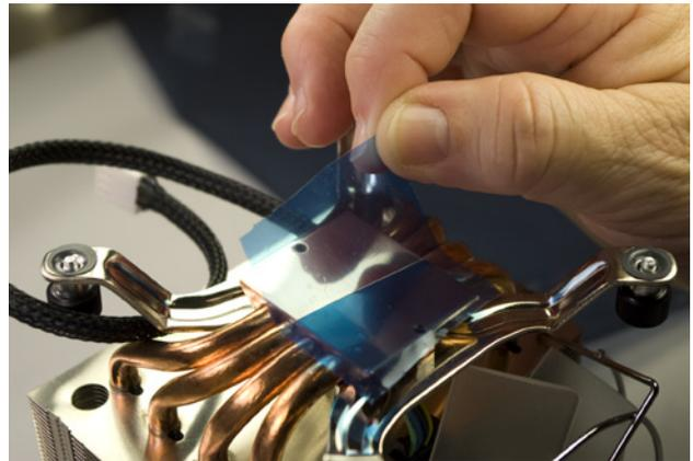
**Figure 5-31.** Peel off the protective plastic film that covers the heatsink base
