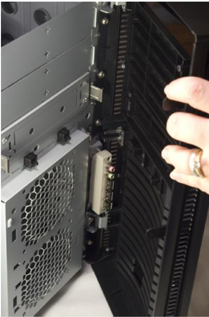
**Figure 8-5.** Swing the front bezel out to about 45°, lift it clear, and set it aside
