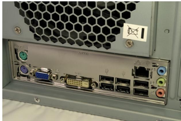
Figure 3-29. Verify that the back panel connectors mate cleanly with the I/O shield
