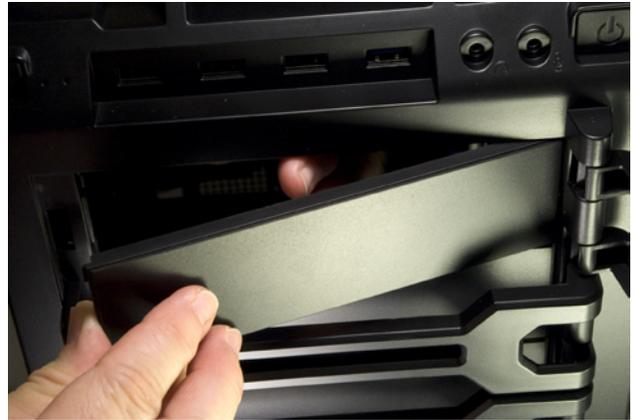
**Figure 5-60.** Snap out the plastic drive bezel
