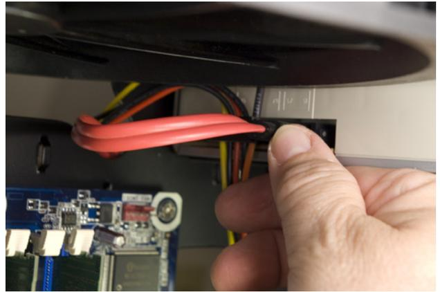
Figure 4-57. Connect a standard SATA data cable to the optical drive
