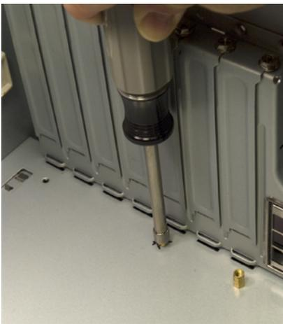
**Figure 8-32.** Install four additional standoffs in the marked mounting holes
