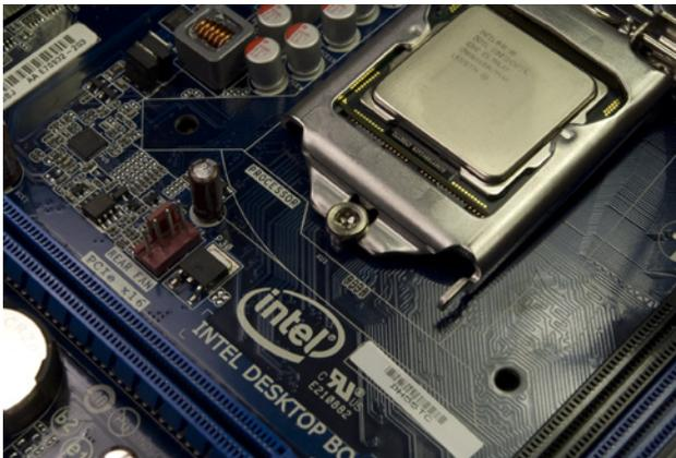
**Figure 6-12.** Lower the processor lever to cam the load plate into locked position
