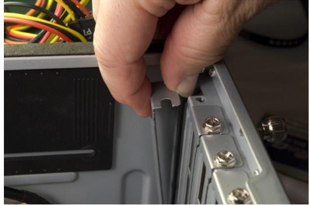
**Figure 6-55.** Tilt the expansion slot cover toward the inside of the case and pull it free
