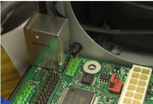
Figure 7-13. Motherboard installation blocked by a protruding connector
