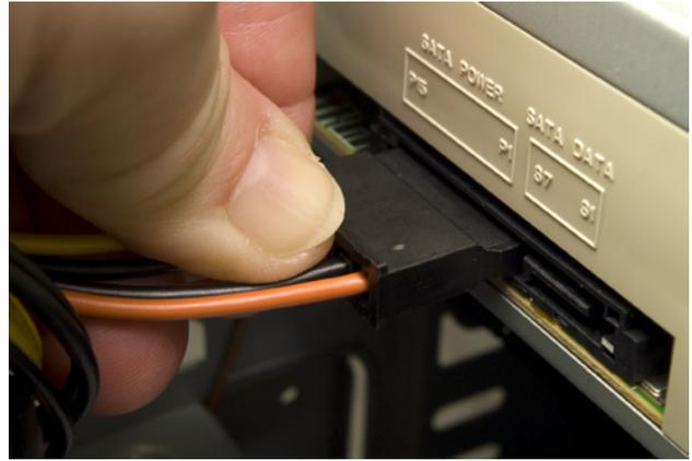
Figure 3-37. Connect a SATA power cable to the optical drive
