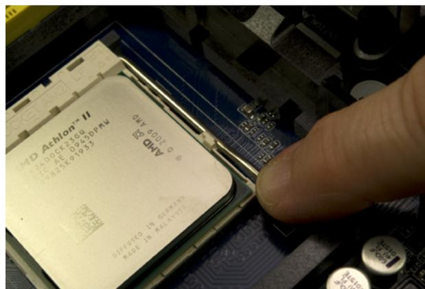
Figure 8-19. Press the cam lever down and snap it into place under the plastic locking tab on the processor socket
