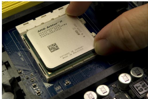
**Figure 3-18.** Orient and align the processor properly with the socket and then drop it into place
