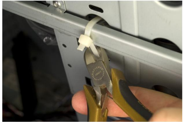
**Figure 8-10.** Cut the cable tie that secures the parts bag to the chassis
