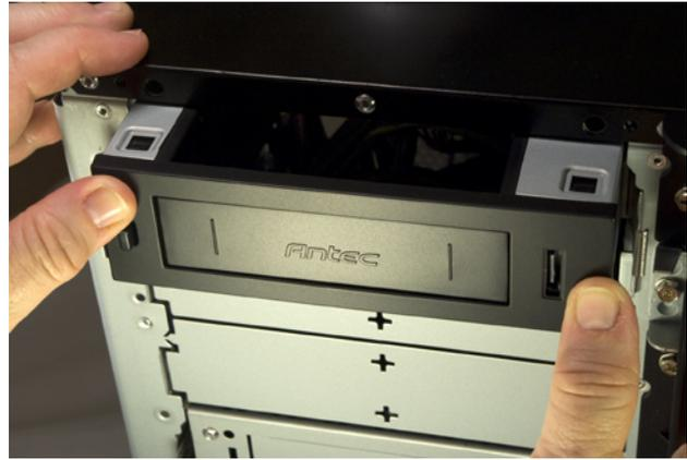
**Figure 8-46.** Installing an Antec Easy SATA hard drive docking station
