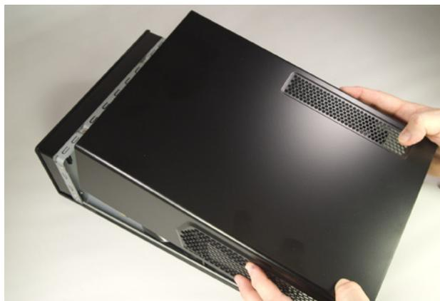
Figure 7-3. Slide the cover back about a third of the way and lift it off
