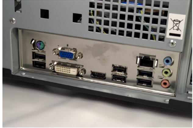
Figure 6-24. Make sure the back-panel connectors mate cleanly with the I/O shield
