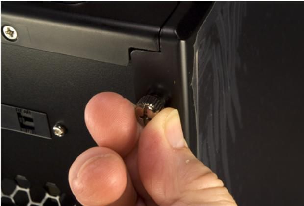
**Figure 4-2.** Remove the top and bottom thumbscrews from the right side panel
