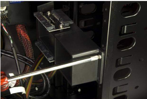
Figure 5-51. Removing a Fleet-Swap drive bracket
