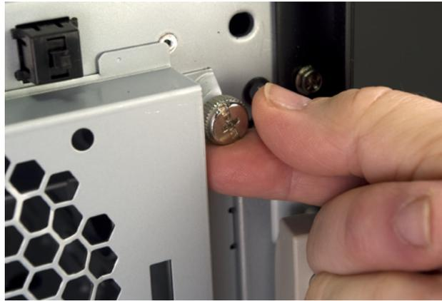
**Figure 8-8.** Loosen the two thumbscrews that secure the hard drive cage cover
