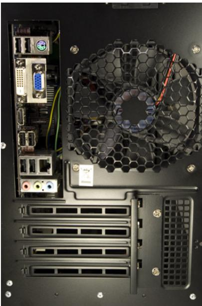
Figure 4-36. Leaving out the I/O shield doesn't greatly increase the open area of the Antec Mini P180 case
