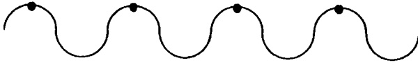
Figure 4.1 If your DVM samples at a frequency related to an AC component of your waveform, you may get false readings.
