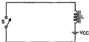
Fig. 85—Simplest form of deflection circuit.
