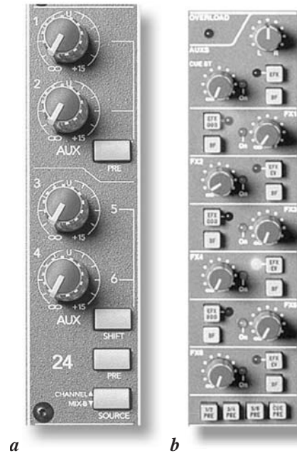
Figure 11.11. Auxiliary send section: (a) Mackie 8-bus (courtesy of Loud Technologies, Inc., www.mackie.com ); (b) Solid State Logic XL 9000 K (courtesy of Solid State Logic, www.solid-state-logic.com ).
