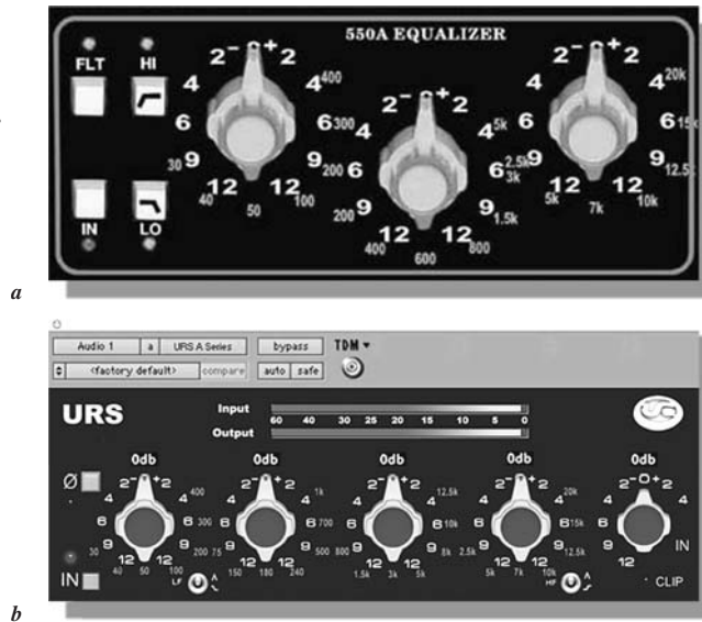
Figure 12.17. The selectable frequency equalizer: (a) venerable API 550A switchable equalizer within the 7600 outboard module (courtesy of API Audio, www.apiaudio.com ); (b) plug-in emulation of the API 550B for TDM, RTAS, and AudioSuite (courtesy of Unique Recording Software, www.ursplugins.com ).
