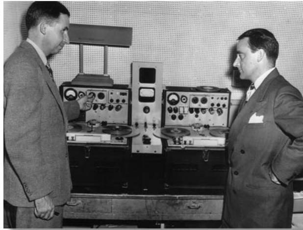
Figure 5.1. John T. Mullin (on the left) proudly displaying his two WWII vintage German Magnetophones, which were the first two tape-based recorders in the United States. (Courtesy of John T. Mullin.)
