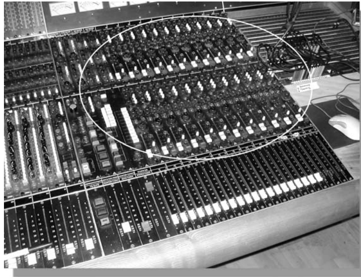
Figure 11.18. Older style English consoles may have a separate monitor section (circled), which is driven by the console's multitrack output and/or tape return buses. (Courtesy of Buttermilk Records, www.buttermilkrecords.com .)
