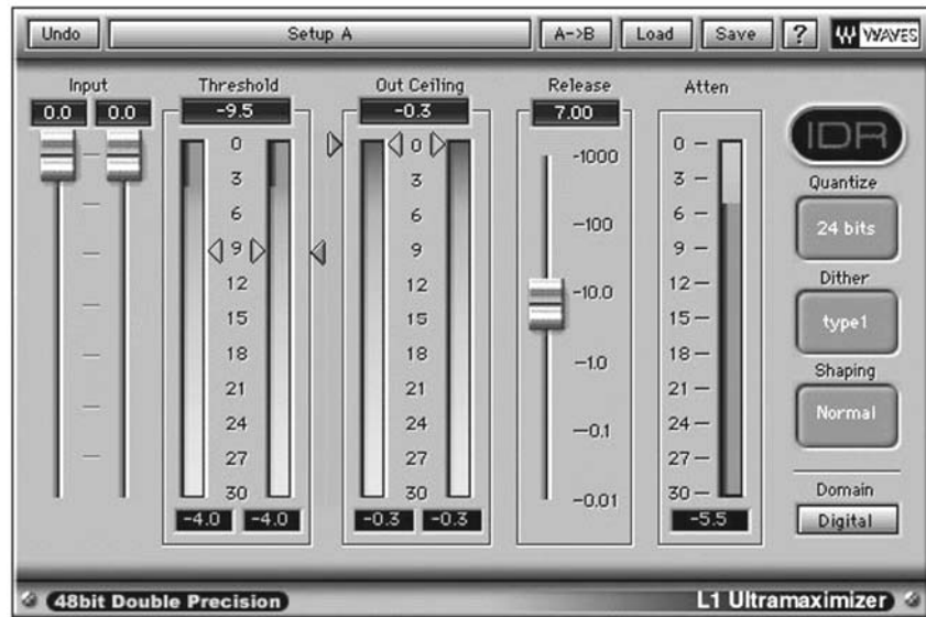
Figure 12.28. Waves L1 Ultramaximizer Limiting/ Quantization plug- in. (Courtesy of Waves, Ltd., www.waves.com.)
