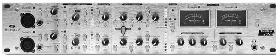
Figure 4.25. Focusrite Platinum TwinTrack Pro dual mono/stereo tracking device. (Courtesy of Digidesign, a division of Avid Technology, Inc., www.digidesign.com .)
