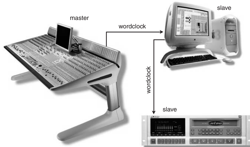
Figure 6.22. Example of wordclock distribution showing that, within a digital production network, there can be only one master clock.
