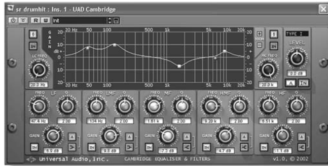
Figure 16.4. Cambridge EQ plug-in for the UAD-1 card. (Courtesy of Universal Audio, www.uaudio.com .)
