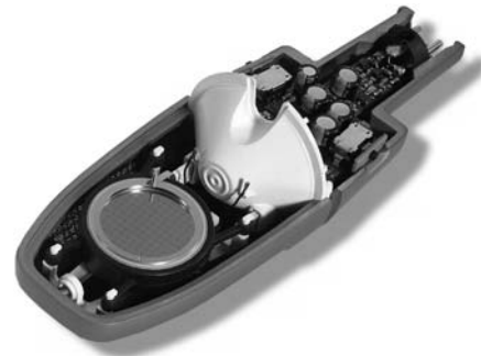
Figure 4.7. Inner detail of an AKG C3000 B condenser microphone. (Courtesy of AKG Acoustics, Inc., www.ake.com .)
