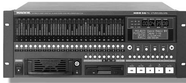
Figure 6.37. Mackie HDR 24/96 multitrack hard disk recorder. (Courtesy of Loud Technologies, Inc., www.mackie.com .)
