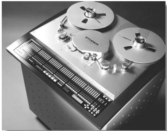
Figure 6.26. The Studer D 827 Mark II MCH 24-/48-track digital audio multitrack recorder. (Courtesy of Studer Professional Audio AG, www.studer.ch .)
