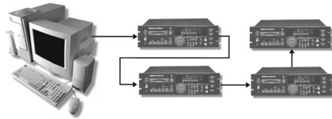
Figure 6.19. Digital audio can be distributed in a daisy-chain fashion.
