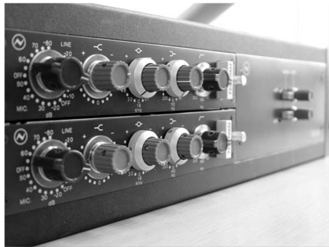
Figure 16.3. Neve 1073 outboard EQ rack. (Courtesy of AMS Neve plc, www.ams-neve.com .)
