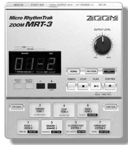
Figure 7.35. Zoom MRT-3B Micro Rhythm Trak Drum Machine. (Courtesy of Samson Technologies Corp., www.samsontech.com/zoom/ .)
