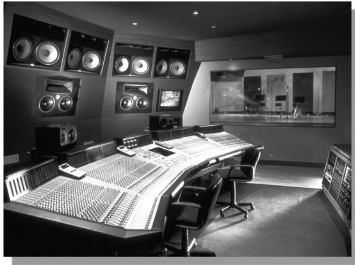
Figure 14.1. Example of a professional monitoring system. (Mega Studios, Paris. Courtesy of Solid State Logic LTD., www.solid-state-logic.com .)
