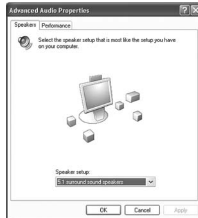
Figure 8.6. Windows XP speaker setup box for stereo, surround, and other playback schemes.
