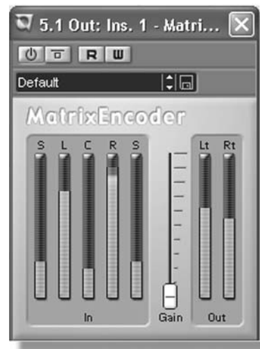
Figure 15.10. Steinberg's Matrix Encoder is capable of encoding a discrete surround mix into a phase-encoded surround form. (Courtesy of Steinberg Media Technologies GMBH, www.steinberg.net .)
