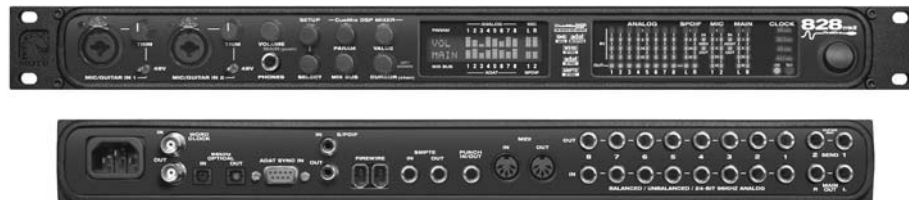
Figure 6.56. Mark of the Unicorn 828 mkII FireWire interface. (Courtesy of MOTU, Inc., www.motu.com .)
