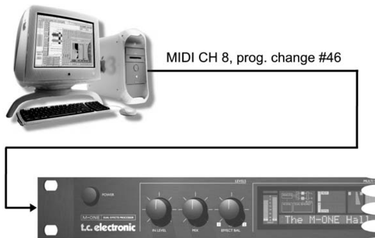
Figure 12.49. Effects settings can be automated throughout a system with the use of MIDI program-change commands.
